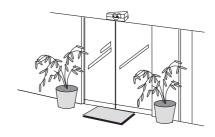
5. Sensing hole must face the bottom, or the sensor doesn't operate normally.
